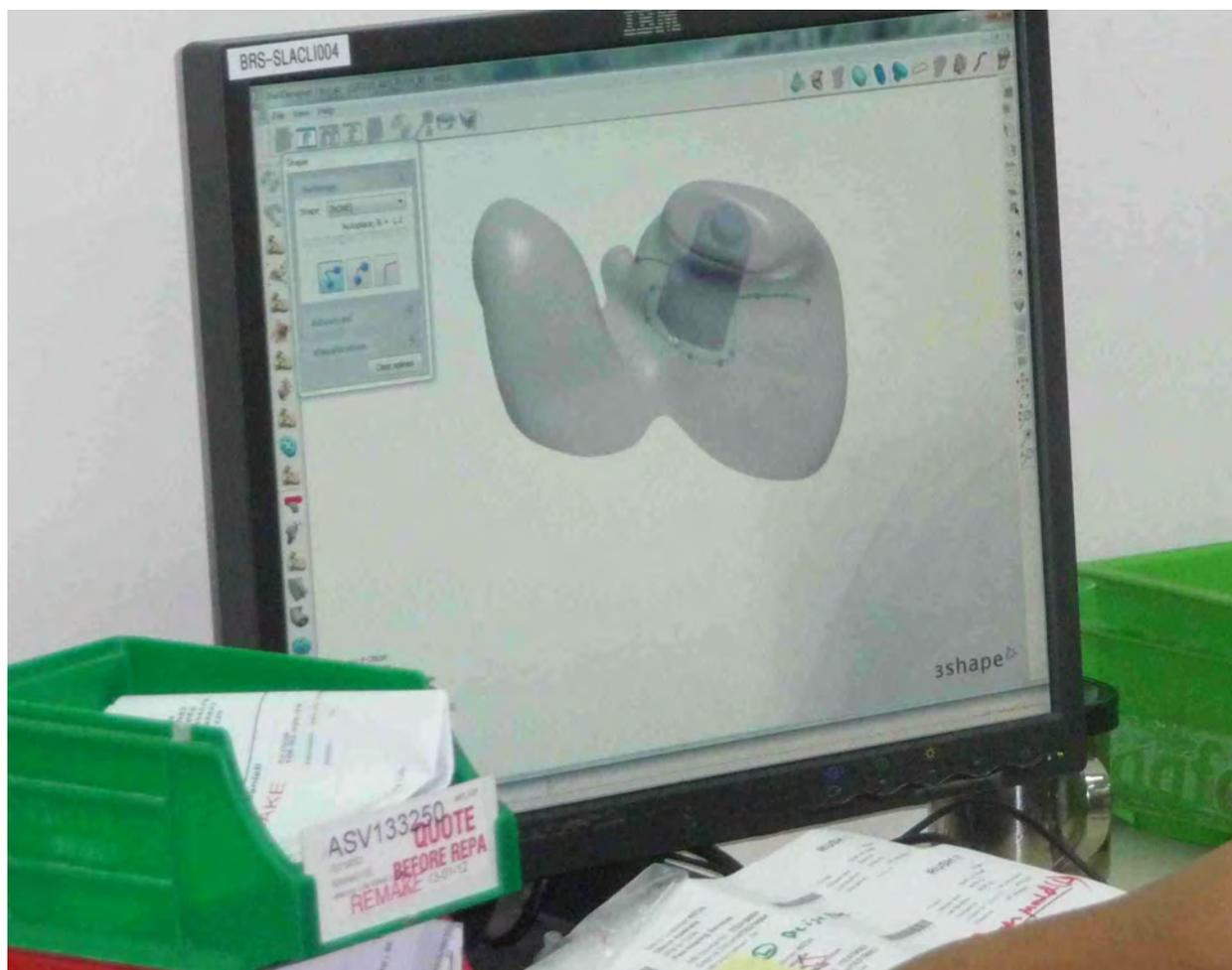
... all the components are to scale, to actual size, and it's just placing them until they go green with a bit of allowance or space each side for various things. ... if the components are green that means they're okay. They're not squashed together, they're not going to cause feedback and things, and there's adequate room for the assemblers to put the physical in reality components inside the shell. (Bert)
